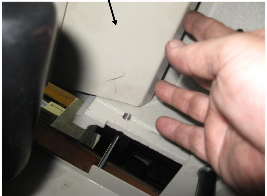
Thread the handle into the block on the right hand side of
